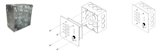
**Note:** If mud rings are used - they may vary slightly depending on the manufacturer and depth of the ring itself. It may be necessary to modify the corners of the mud ring for proper fit. The corners on the mud ring as shown below right have a larger radius than the one on the left and will need a bit of filing for the Mini wall controller to fit. (The Appleton ½" mud ring shown at the left below will fit without modification)
