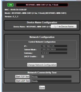
In the **Network Properties** window that opens as shown at the left - select **“Change Network Configuration”** in order to disable DHCP and to insert IP addresses manually (it also provides two built in test procedures, device security, and device information).
