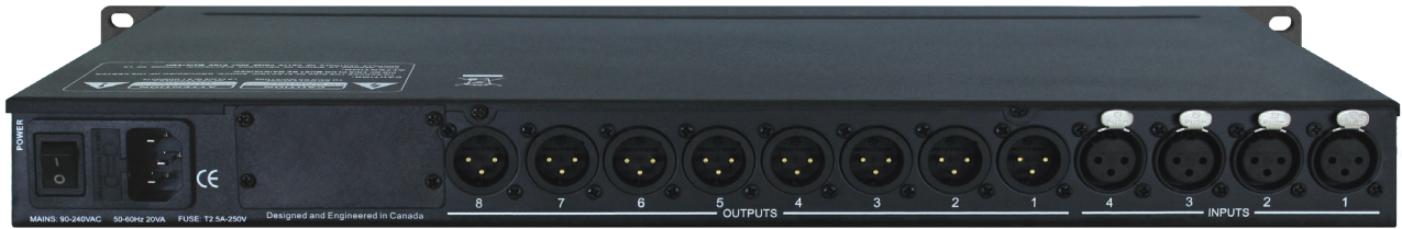
Rear panel view of the XA-4080, with XLR I/O section.
